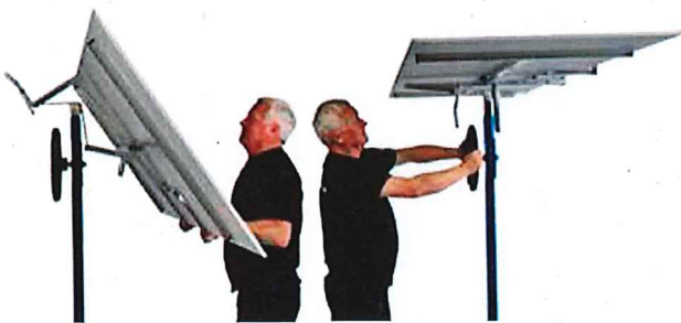
Raise the board and angle the load carrier to the desired angle. Then raise using the knob.
